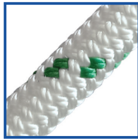
Q5176 10MM YACHT BRAID BREAKING STRENGTH: 2200KG CONSTRUCTION: POLYESTER
